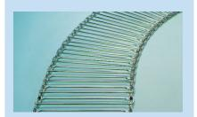
The galvanized conveyor chain consists of two tempered external chains with rods welded in between. The horizontal rods are placed at an even level to ensure that eggs are gently placed on the conveyor, can easily make their way through transfer areas and are not crushed on the inside of bends. Please see the information sheet "Conveyor Chains" for details concerning the appliable conveyor chain angles.
